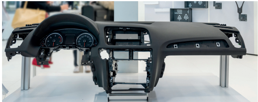
Fig. 4. The pretreatment with plasma makes non-polar plastics susceptible to adhesion processes and ensures a firm connection of the different, sometimes even incompatible materials, for example when laminating dashboards made of recycled materials with powder-sintered molded skins made of soft plastic. © Plasmamatreat
