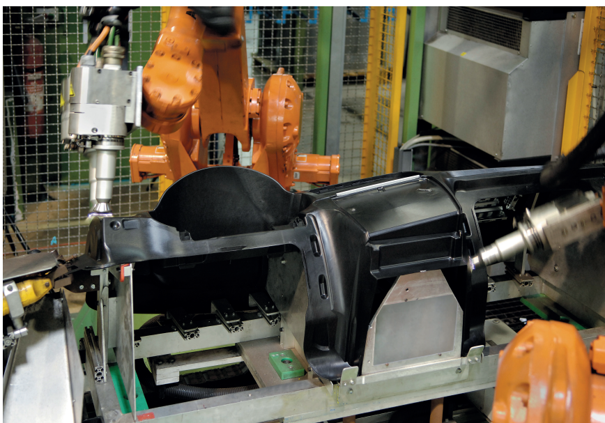
Fig. 5. Activating the surface with plasma technology increases the surface energy and improves the adhesion of adhesives and paints, even with plastic parts made from recycled material. © Plasmamatreat
